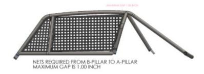
**Window Nets** - Window nets are required from B-Pillar to A-Pillar and that the maximum gap is one (1) inch.
